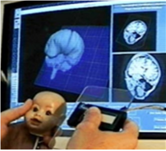
Figure 4: Three-dimensional props to control the cutting plane location: [13]
